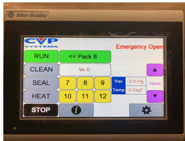
Figure 3-1. Emergency-Open switch is applied
