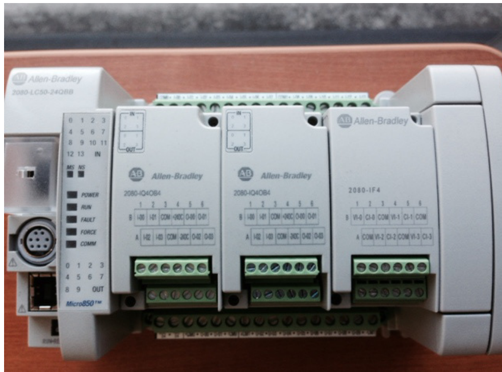
Figure 11-1. Status Lights on the PLC
