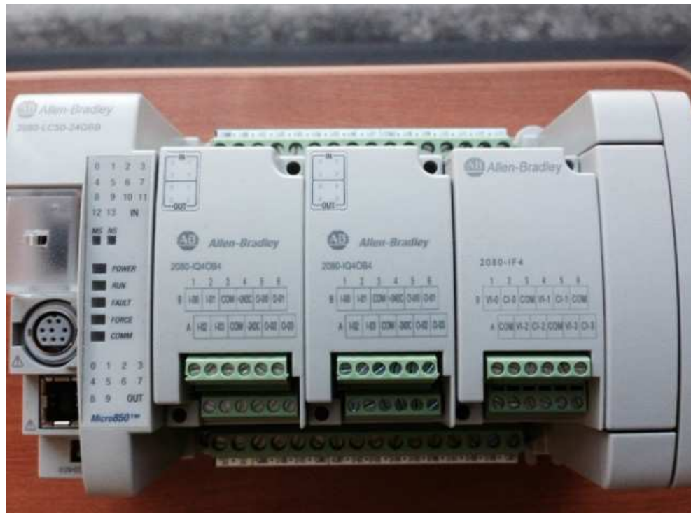
Figure 11-1. Status Lights on the PLC
