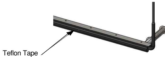
Figure 10-7. Teflon Tape on the Heat Seal Bar
